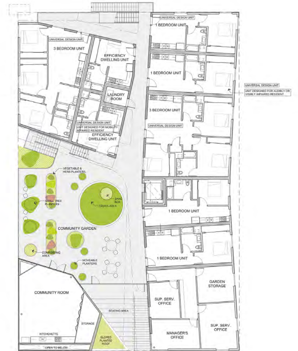
The MLK1101 project (Los Angeles) includes several types of apartments. For example, some apartments are fully accessible, while others have a different number of rooms. A variety of exterior and interior spaces allow PEH to enjoy activities as they wish. (see practice 5.3 a), p. 66)
